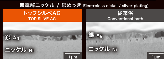
無電解ニッケル / 銀めっき後の断面SIM像 SIM image of cross section(after electroless nickel/silver plating)
