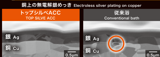
無電解銀めっき後の断面SIM像 SIM image of cross section(after electroless silver plating)
