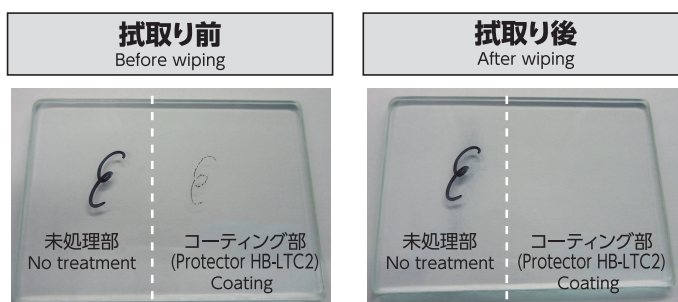
油性マジックの拭取り試験 Oil-based marker wipe-off test
