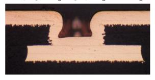
Current density: 3 A/dm² via diameter 140 μm, via depth 80 μm
