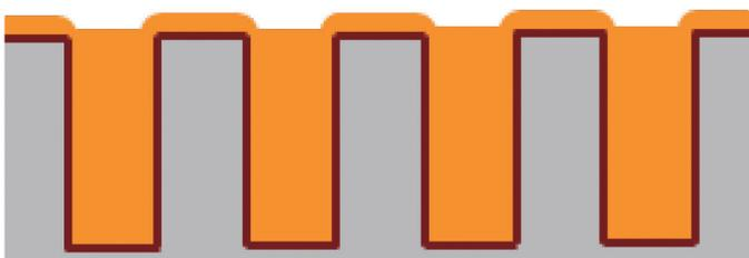
Aperture diameter 50  $\mu\text{m}$ , via depth 55  $\mu\text{m}$
