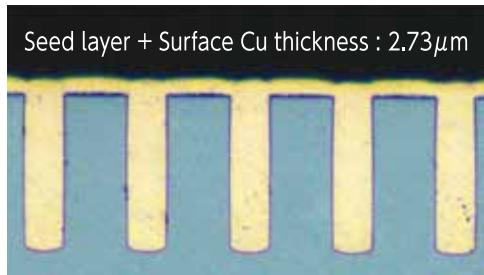
Current density : 0.2A/dm<sup>2</sup>, via diameter : 7μm, via depth : 25μm
