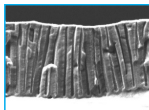
陽極酸化皮膜断面SEM像 多孔質な酸化皮膜を形成 Cross-sectional SEM image of an anodic oxide film Formation of porous oxide film
