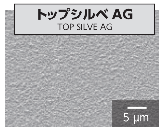
無電解銀めっき後の表面 SEM 像 SEM image of surface (after electroless silver plating)
