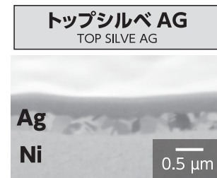
無電解ニッケル / 銀めっき後の断面 SIM 像 SIM image of cross section (after electroless nickel/silver plating)
